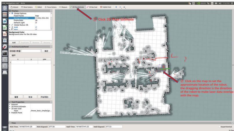
After setting the positioning, the laser shape and the scene shape in the map have basically overlapped, the means the regulation is complete. As the picture shown below.
