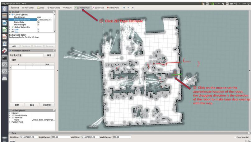
After setting the positioning, the laser shape and the scene shape in the map have basically overlapped, the means the regulation is complete. As the picture shown below.
