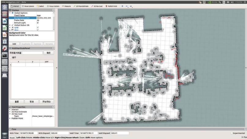
(4) Set multiple target points on the multi-point navigation plug-in in the left column, click Start Navigation, and switch the SWB to command control mode.
