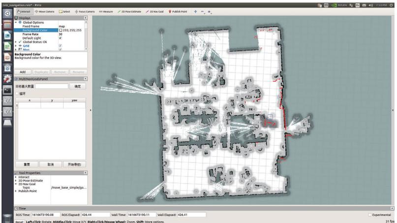
(4) Set multiple target points on the multi-point navigation plug-in in the left column, click Start Navigation, and switch the SWB to command control mode.
